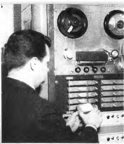
Staff announcer Lou Sherman places into position a MacKenzie Cartridge. The electronic tape machine expedites radio operation for spot announcements.
