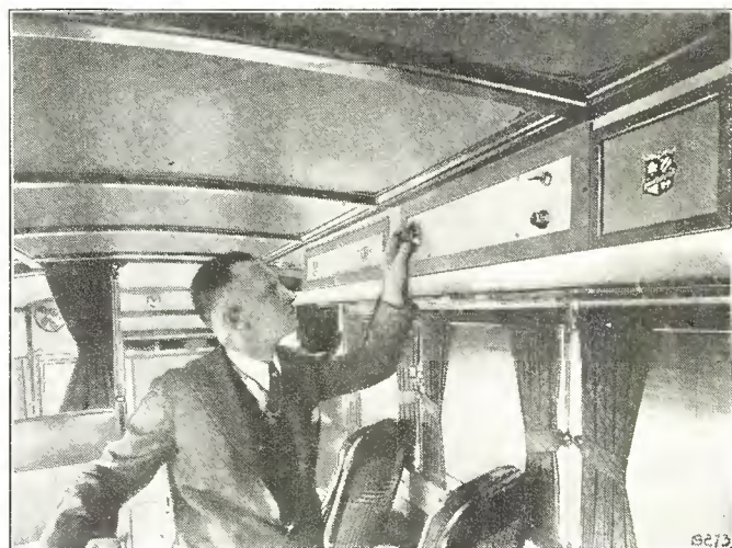
Installed in locker compartments above the seats the Delco standard set is easily accessible for tuning. This photo shows the interior view of the Bonne Entente II used by GM executives while travelling in Canada. The receiver has automatic volume control to compensate for variations in signal strength
