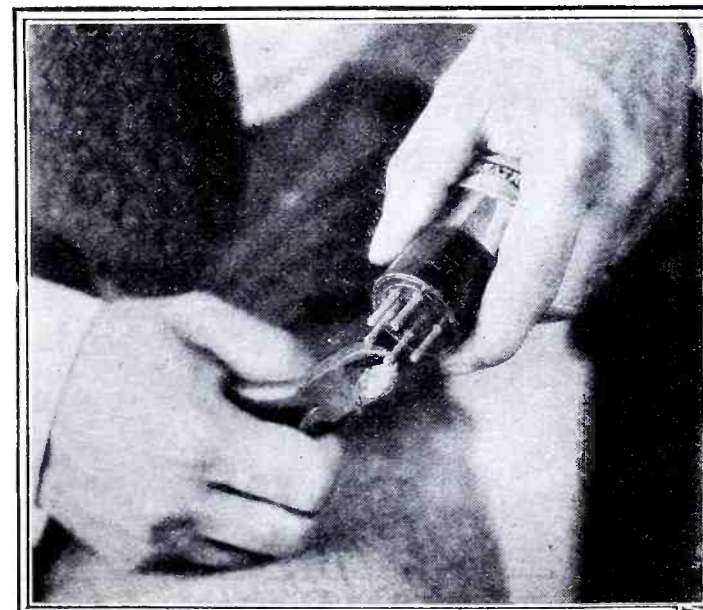
Where springs in tube sockets do not make electrical contact with the tube prongs on account of oxidization, a pair of diagonal cutters, as shown above, may be used to cut a ring around the end of each prong. This ring, being raised, cleans off contact corrosion when the tube is worked up and down in the socket.
