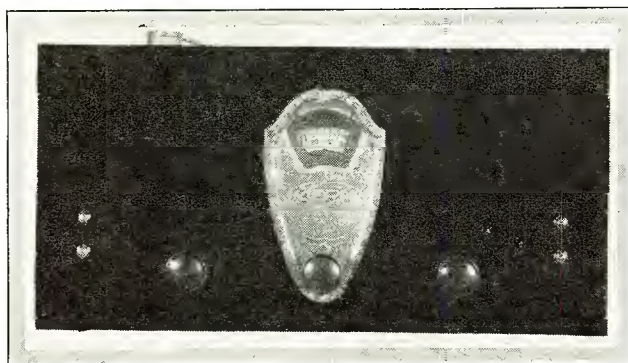
Fig. 2. The front panel view of the receiver is shown in the above photograph. The knob at the left controls the regeneration condenser, while the central knob is the one of the drum dial. The knob at the right is the combined 20 ohm filament rheostat and filament switch
