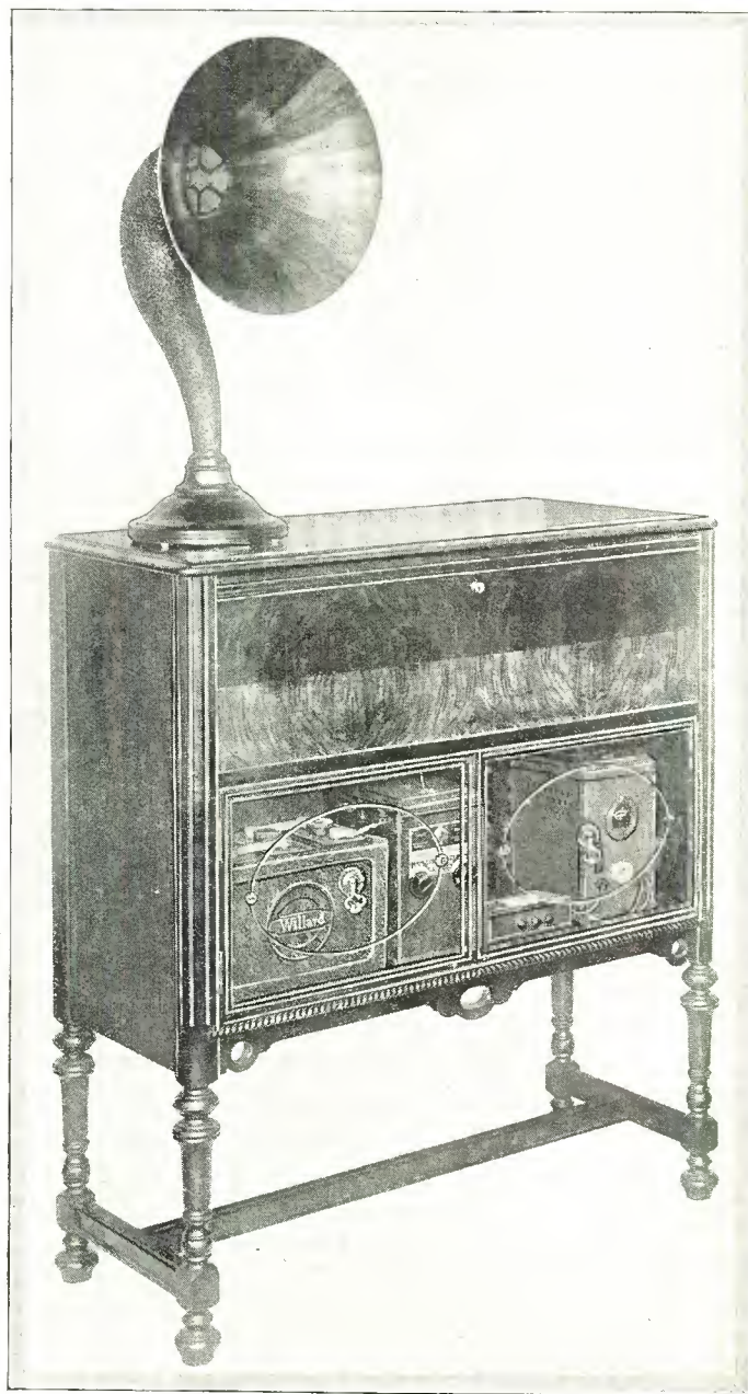
View showing the completed receiver installed in a console with accessories
