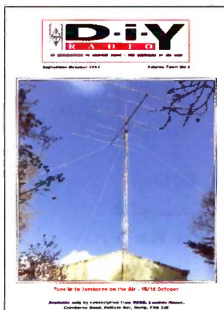
COVER PICTURE: The six element multiband antenna and mast used at the JOTA special event radio station GB4AGG.
