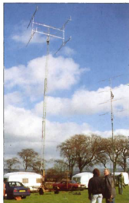
The antennas up in the air - left: 144MHz on trailer tower, right: 432MHz on pneumatic mast.
