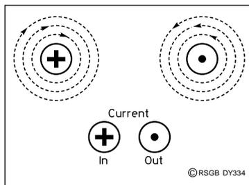
Fig 1: Concentric magnetic fields around a conductor carrying current.
