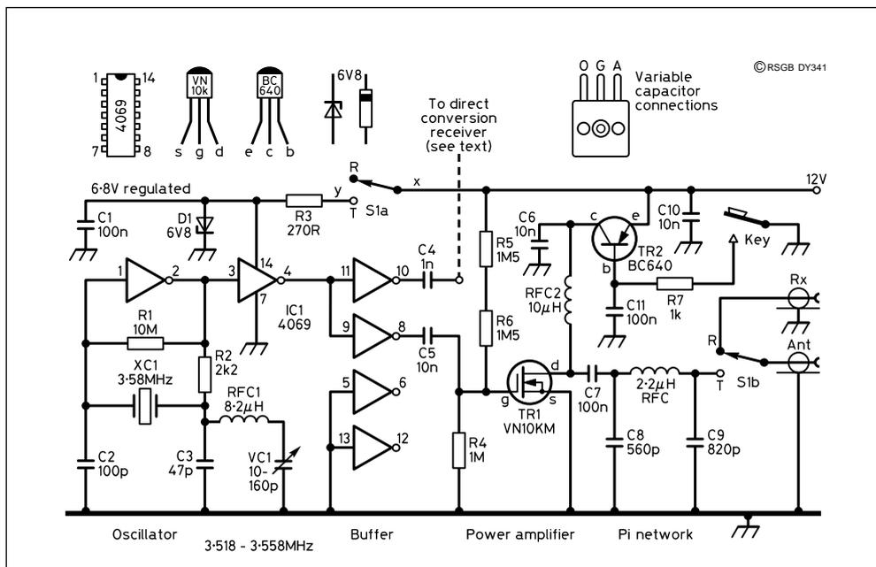
Fig 2: Circuit diagram of 80 metre transmitter.
