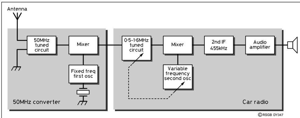
Fig 1: Block diagram of the 50MHz receiver
