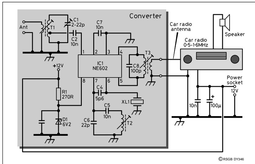
**Fig 2: Circuit diagram of 50MHz receiver**
