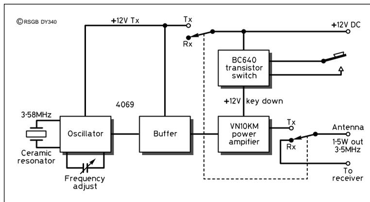
Fig 1: Block diagram of the ceramic resonator controlled 80m CW transmitter.
