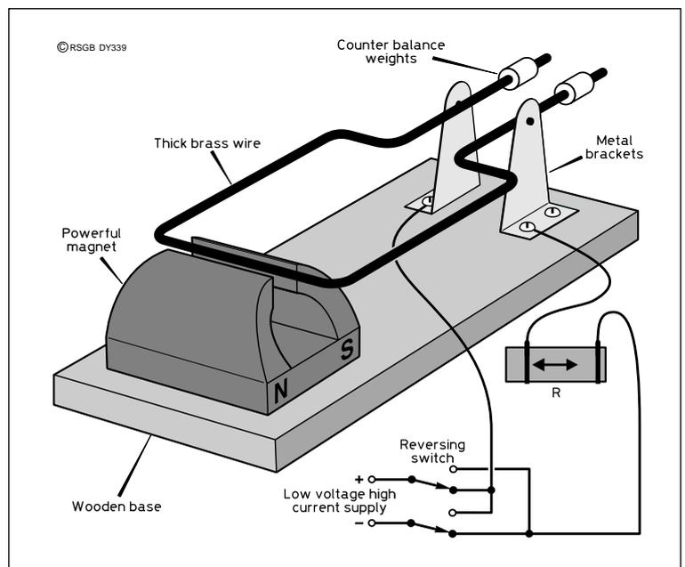
Fig 5: Magnetic balance for measuring current.
