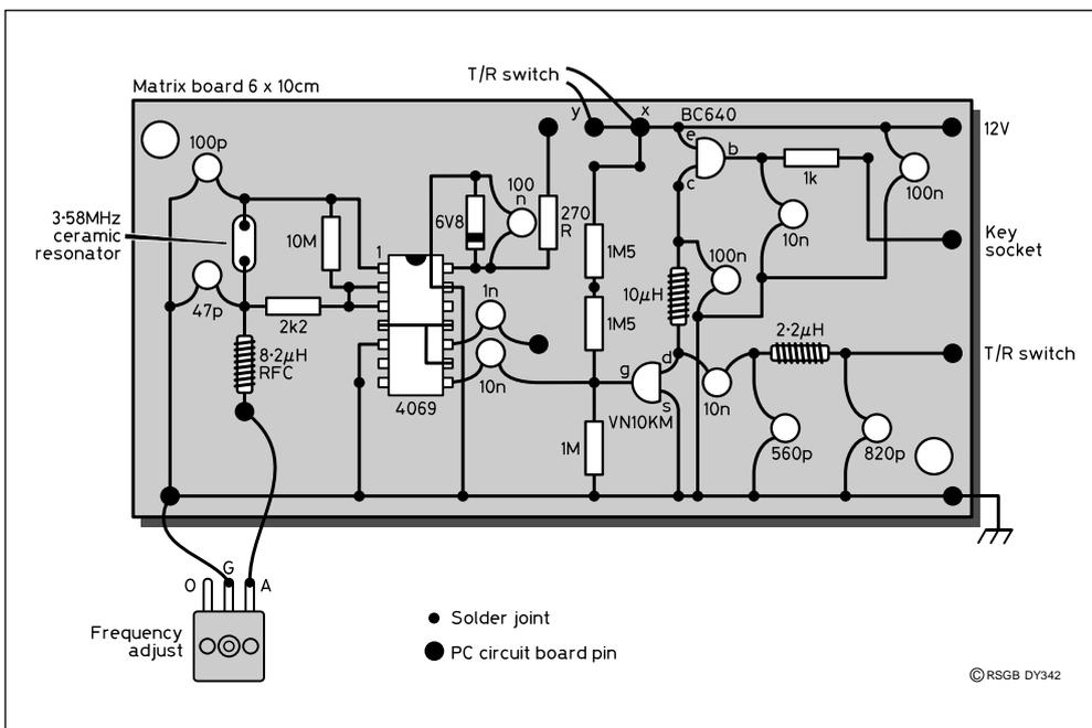
Fig 3: Component layout of the 80 metre transmitter. The Transmit/Receive switch is not mounted on the board and is not shown in this diagram.
