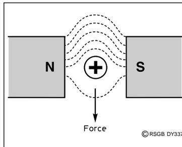
Fig 4: Interaction of a conductor carrying current and a magnetic field.
