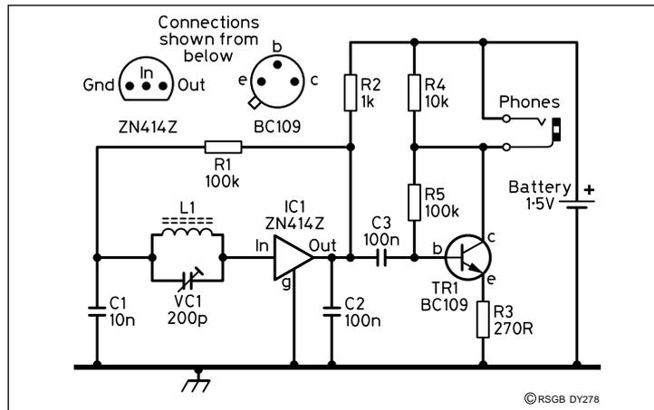
Fig 1: Simple medium-wave radio, circuit diagram. Note that the pin connections to IC1 and TR1 are shown from below.
