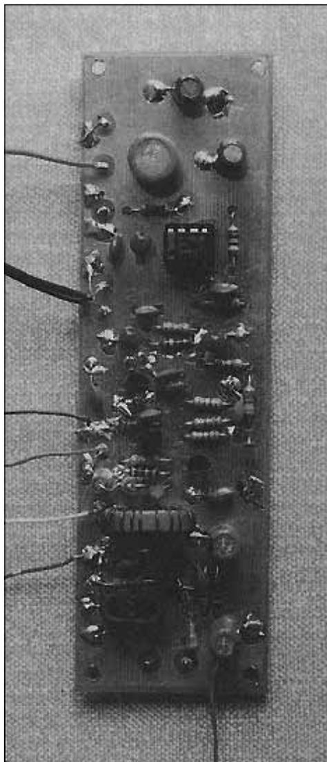
The Nicky is simple to assemble on a printed circuit board.
