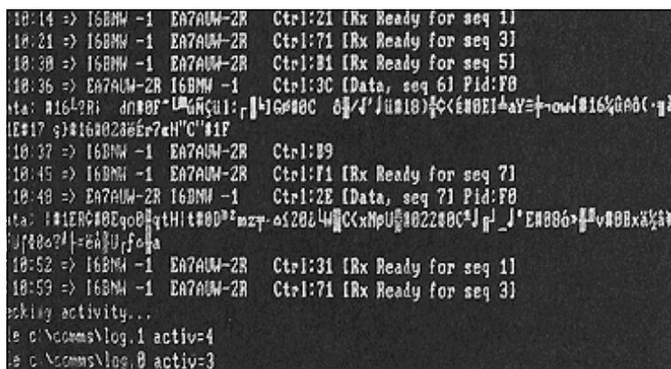
Fig 3: Detail of the PKTMON screen showing accurately received packets but unreadable 'data' lines. The lines starting with c:\comms\log report on which files are collecting the data.
