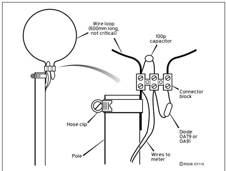
Fig 2: Broadband and tunable field strength meter.
