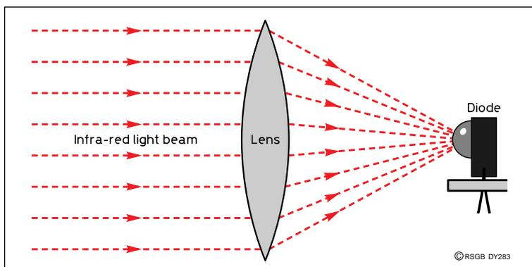
Fig 2: A simple lens focuses the infra-red light to improve the signal.
