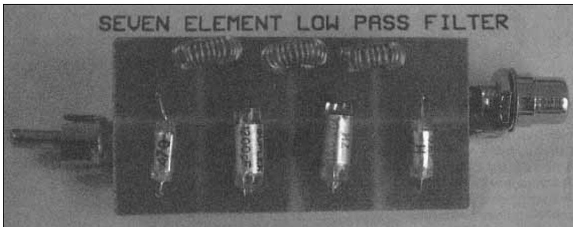
Filter components soldered to PCB board pads.
