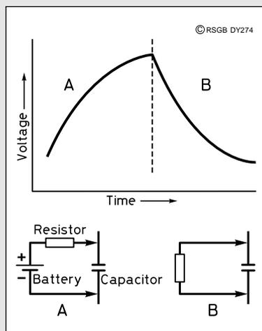
connected across a resistor (see B) current will flow through the resistor and discharge the capacitor. The capacitor's voltage now drops - see curve B. The higher the value of the resistor, the longer it takes to charge, or discharge, the capacitor.
