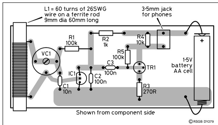
Fig 2: Component layout using PCB board.
