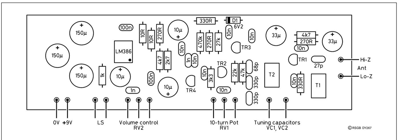
Fig 3: Layout of the Nicky receiver circuit board.
