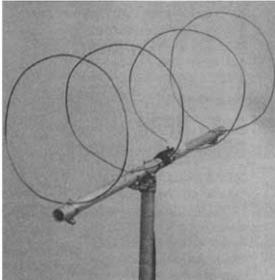
antenna uses wire loops. This is a very well known antenna in amateur radio and it is called a **quad**. Normally, these wire loops are square. For the lower frequency bands the elements are much larger and have to be supported on an X frame. In our case a quad antenna for 432MHz is very small so the elements do not need a supporting frame and can be made in a circular shape.
