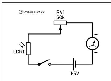
Fig 1: Circuit diagram of photometer.
