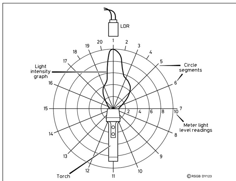
Fig 2: Torch light intensity pattern plotted at RSGB HQ.
