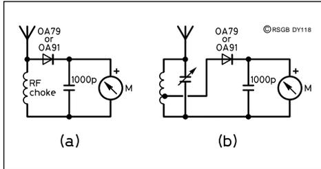
Fig 1: Construction of the UHF field strength meter.
