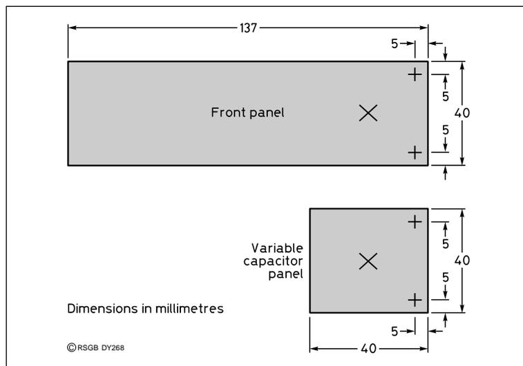
Fig 4: The case can be metal or made from PCB material.
