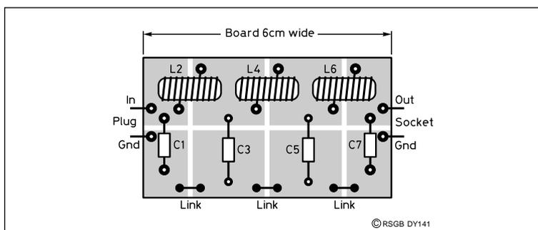
Fig 2: Layout and construction of filter.
