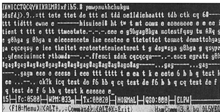
Fig 1: Detail of the HamComm Morse receiving screen. Some callsigns are visible, especially the CQ call from a French station at the bottom. Note the printed dashes and dots which appear when the program can't decipher the Morse character.
