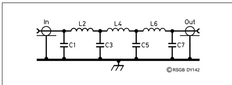
Fig 1: Circuit diagram of filter.
