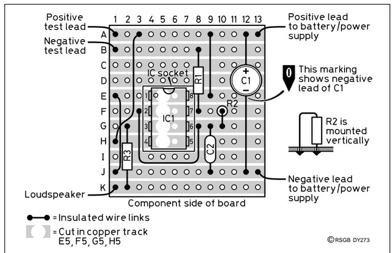
Fig 2: Veroboard Layout for the D-i-Y'er 555. If you can read a circuit diagram, the project can be built using other methods.
