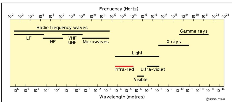
Fig 1: Infra-Red light is lower in frequency than visible light.
