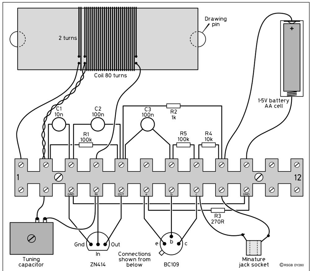
**Fig 3: Component layout using connector strip.** This layout is shown using the plastic or cardboard tube alternative coil former. An external wire antenna can be connected to tag strip connector 1 if required.
