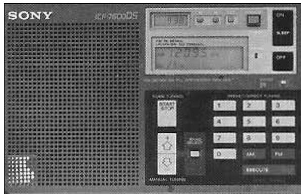
The Sony ICF-7600DS receiver provides digital frequency readout and is used by many for shortwave broadcast listening.
