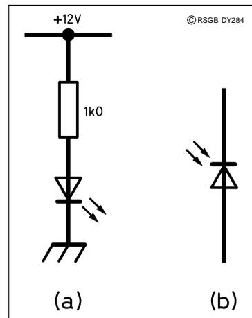
Fig 1(a) LED operating from a 12V supply with a current limiting resistor. Fig 1(b) shows the symbol for a photo diode. Note that the two arrows, representing rays of light, differentiate these special diodes from that of a normal diode.
