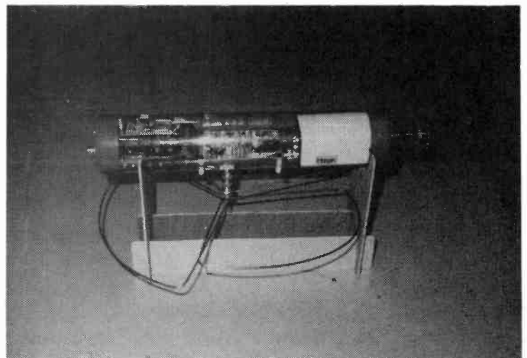
Close-up of the kite ATV payload mounted in the plastic cylinder. An Olde Antenna Labs mini-wheel is mounted below the tube.
