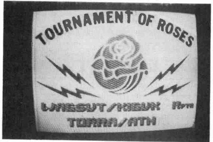
Test pattern from the repeater at Pacific Bell Building in Pasadena. 434 in, 919.25 out.
