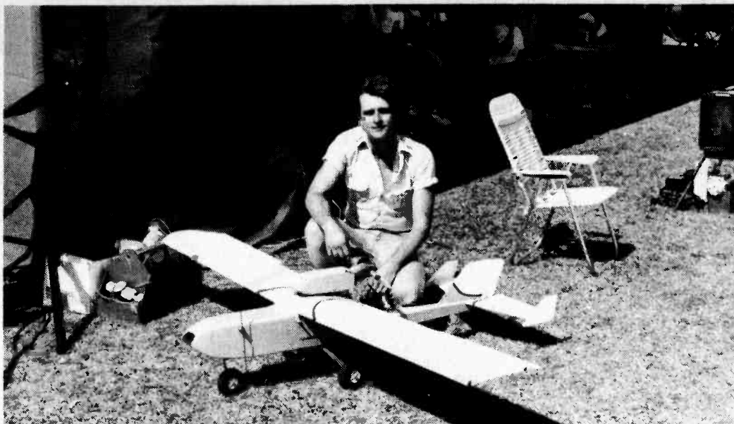
AUTHOR WITH PLANE. ENGINE K&B .61, WEIGHT 13 LBS. WINGSPAN 7 FEET
