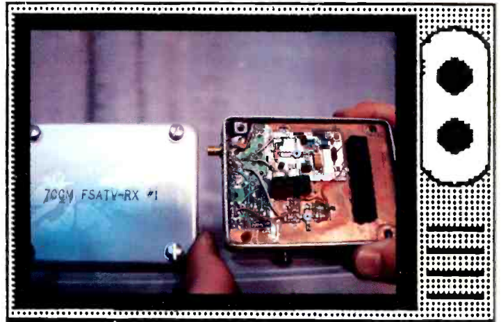
Actual ATV Receiver to be flown on the Space Shuttle for SAREX 90, STS 37.
