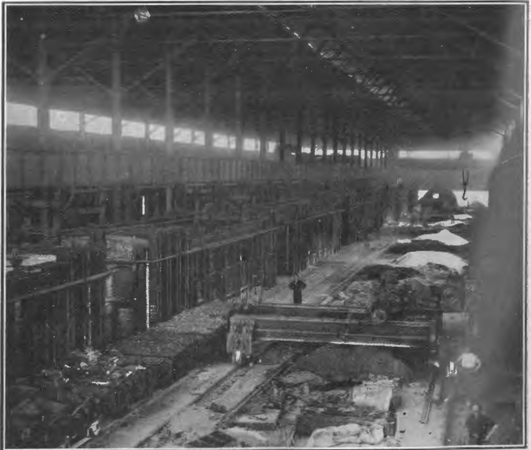
The Open Hearth Steel Furnace House, Showing Raw Materials at Furnace Mouth, also the Electrical Charging Car.
