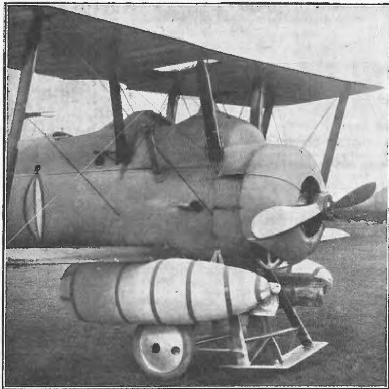
Special Press photo. The floats on the Parnall "Panther" can be inflated by means of compressed air operated from the pilot's seat. When inflated these floats are quite capable of keeping the machine and crew afloat. Photo shows floats inflated.
