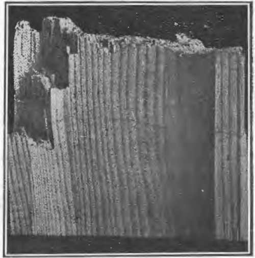
Section of spruce wing beam cut from wood which was broken in the tree, probably when felled.
