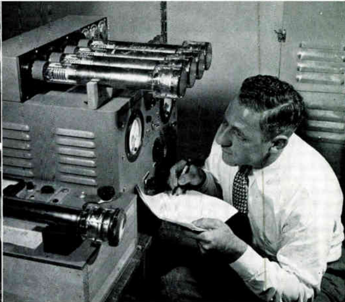
New image orthicon television camera tubes receive a final performance check.
