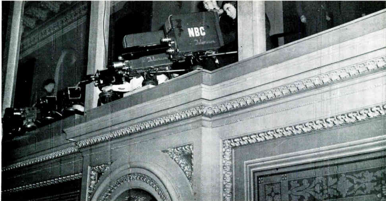
Image orthicon cameras record the opening session of Congress from the visitor's gallery in the House of Representatives.
