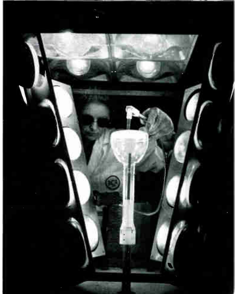
Infra-red lamps dry the fluorescent screen of a television picture tube while being processed.
