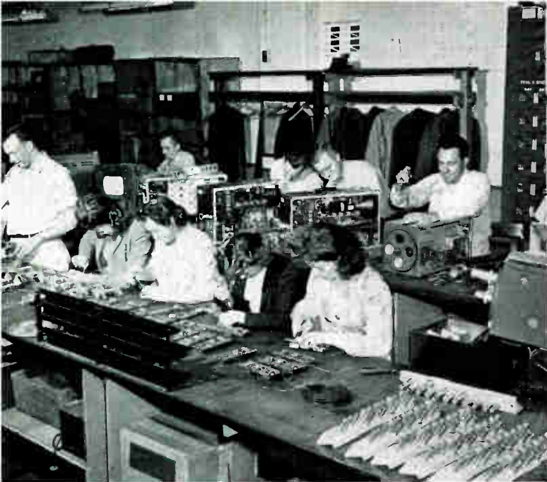
Super-sensitive image orthicon television cameras in various stages of assembly.
