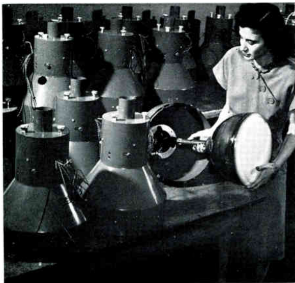
A 12-inch cathode-ray tube for a shipboard radar installation is inserted in its protective metal casing.
