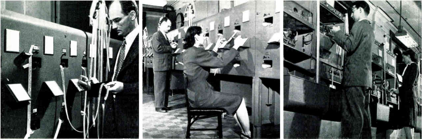
Radiotelegraph messages are received from abroad and transmitted to foreign points through these automatic tape relay machines at RCA Communications, 66 Broad Street, New York.
