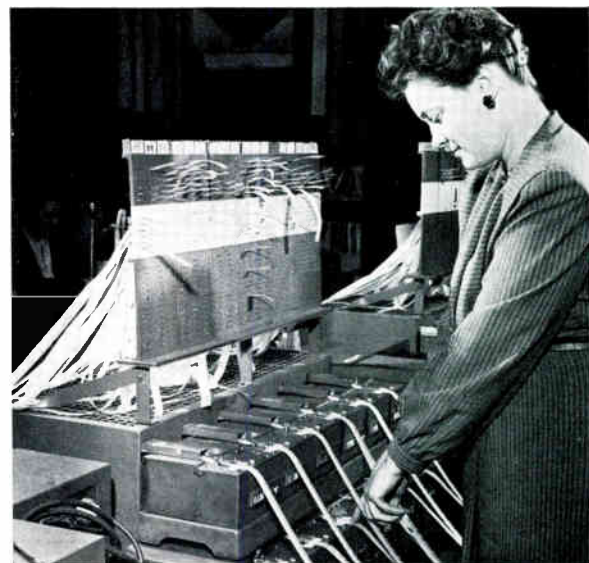
Tapes carrying radiotelegraph messages from overseas are relayed through this machine to their destinations in this country.
