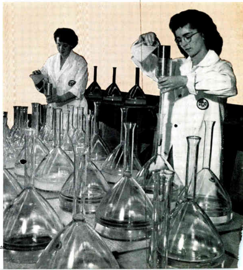
Pouring phosphor solution into television picture tubes to form the fluorescent screens.
