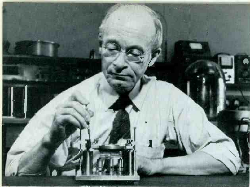
This instrument insures precise placement of tube elements.
