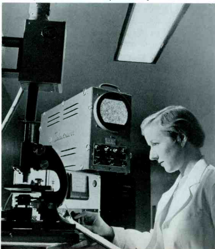
The "Sanguinometer" enables rapid counting of blood cells.
