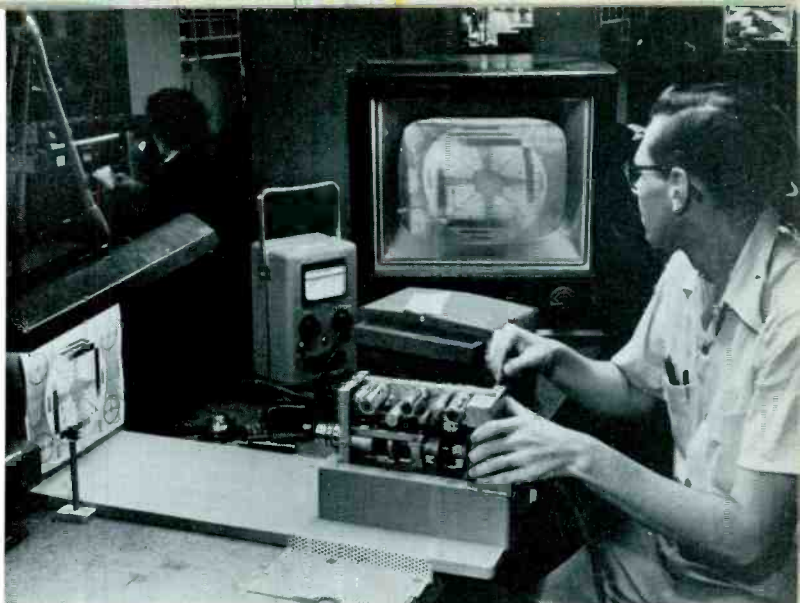
Inspector checks circuits of small "TV Eye" camera.
