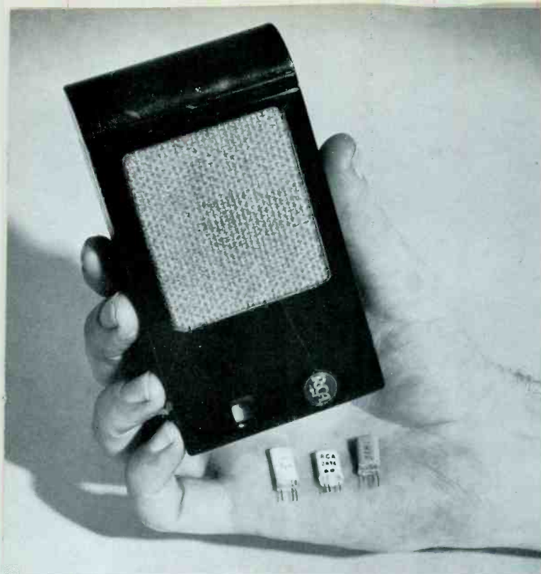
Miniature radio receiver made possible by transistors.
