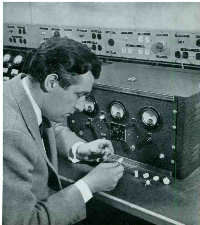
These tiny transistors have built-in cooling systems.
