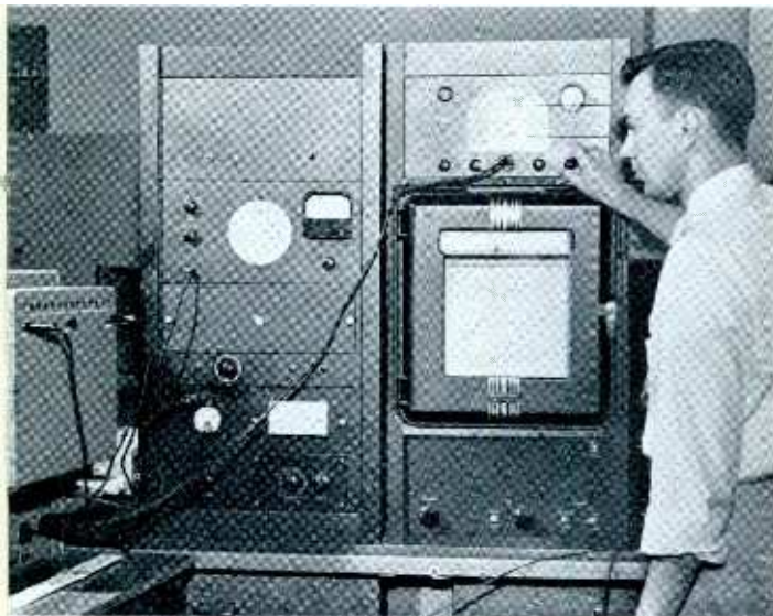
Tonal characteristics of loud speakers are checked and charted by this device.
