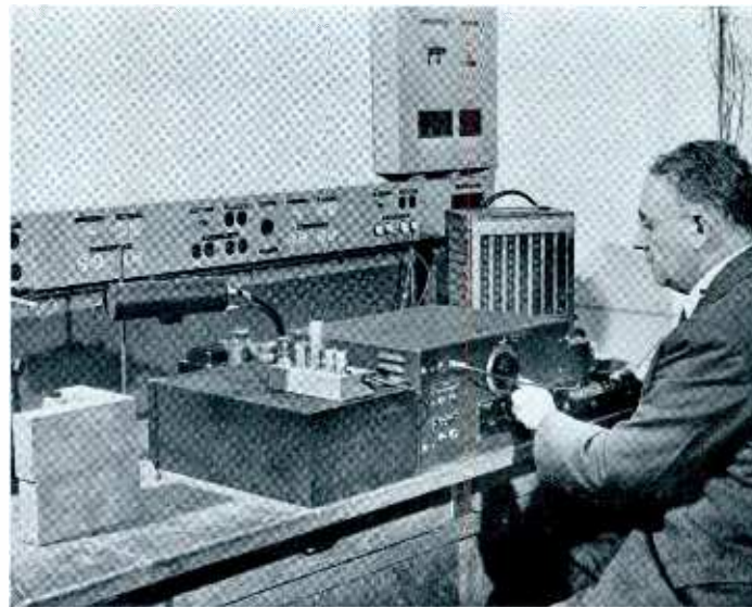
Heart of this scintillation counter is the new RCA multiplier phototube.
