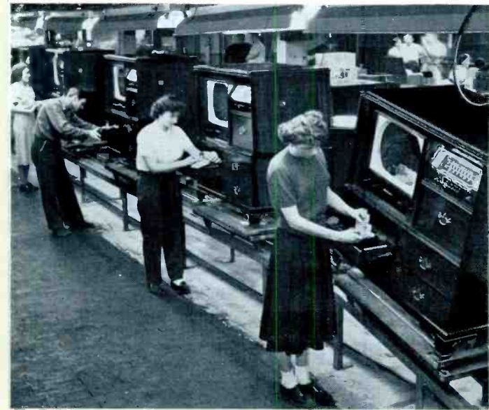
At this section of the Camden, N. J., assembly line, television chassis with 12½-inch tubes are inserted in their cabinets.
