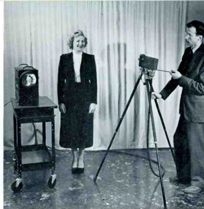
RCA scientist operates a tiny television camera made possible by a newly-developed diminutive pickup tube, the Vidicon.
