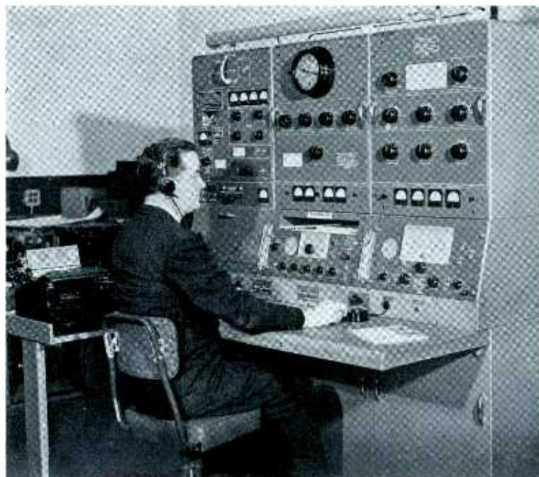
New 500-watt radiotelegraph console designed by Radiomarine for installation aboard luxury liners.
