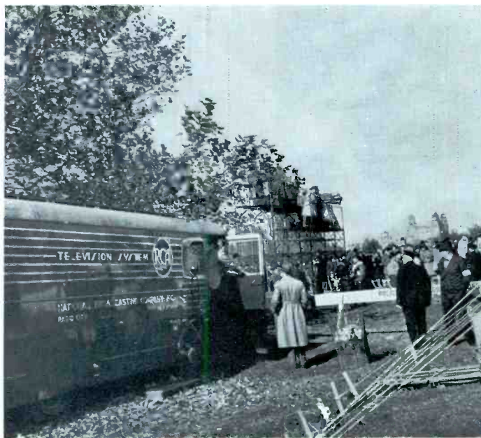
Mobile units make it possible to bring television programs to the main transmitter from remote sports stadia and scenes of news events.
