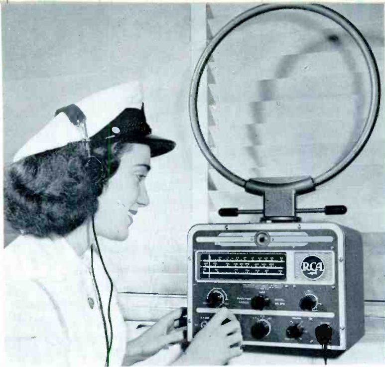
Small-craft radio direction finder with broadcast band auxiliary serves as an accurate navigational aid or a source of entertainment.
