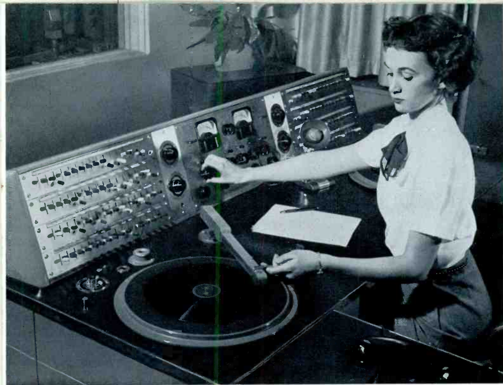
Operator furnishes music to factory employees through this RCA sound distribution system console.
