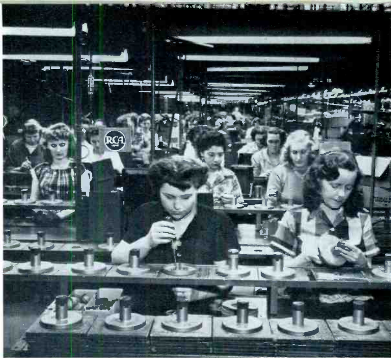
At Indianapolis, 45-rpm turntables are assembled and checked as they move along the production line.
