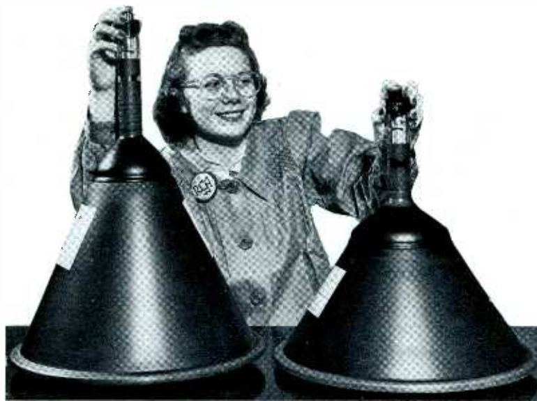
The original 16-inch metal-cone kinescope picture tube is compared with its successor which is approximately six inches shorter.
