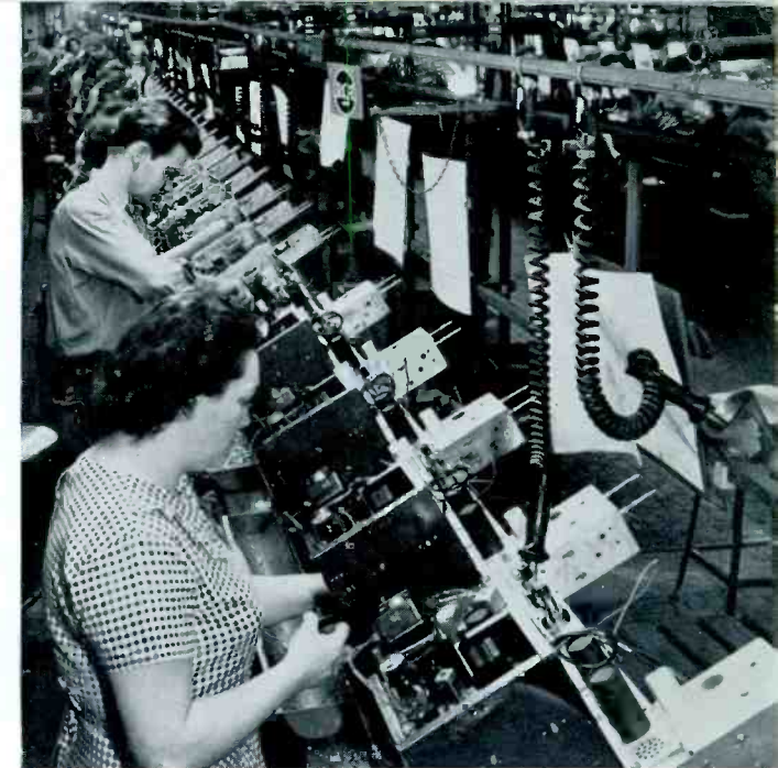
Television chassis move rapidly along the subassembly production line at RCA Victor's Indianapolis, Indiana, plant.
